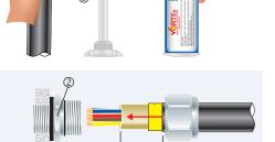
6. Re-insert the barrier pot sub-assembly 5 back into the inner 2.
