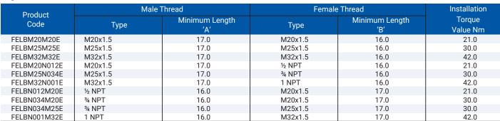
All dimensions except NPT are in mm. For other thread types, contact CCG.
